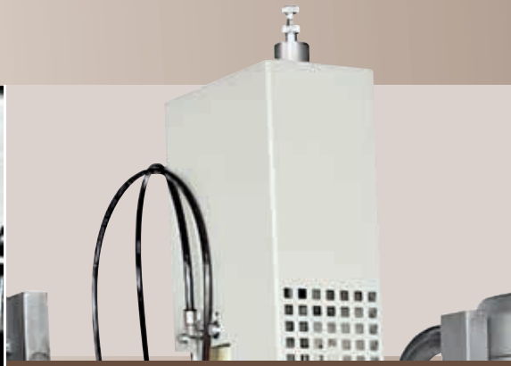
Hydraulic brake for a more precise boring speed control in reduced cycle times (option)
